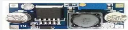
Gambar Module DC Step Down
