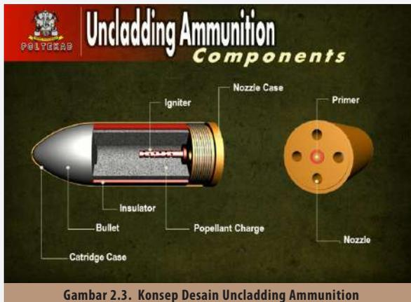
Gambar 2.3. Konsep Desain Uncladding Ammunition
